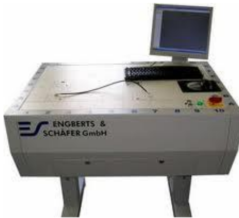
Electrical testing board
